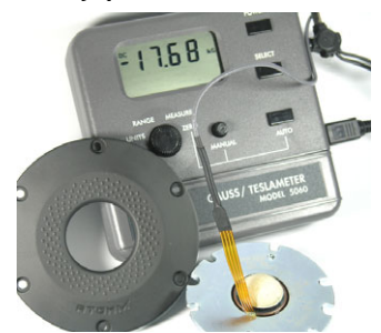
MEASUREMENT OF THE MAGNETIC FLOW USING A PRECISION GAUSSMETER
