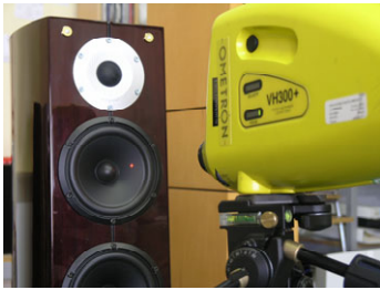
MEASUREMENTS BY LASER VIBROMETER
