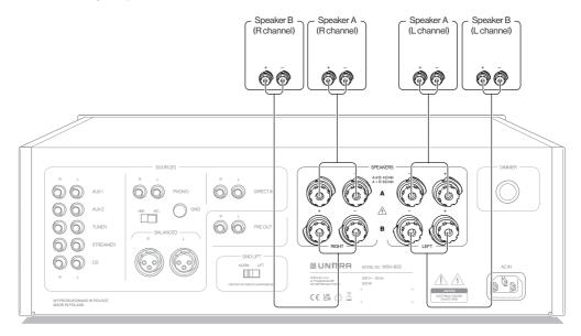
To select a pair of connected speakers, set the SPEAKERS selector switch to A or B. 🖰 p. 8
