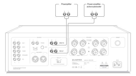
To select the preamplifier connected to the DIRECT IN jacks as the input source, set the DIRECT IN switch to the ON position.  $\stackrel{\triangle}{\longrightarrow}$  p. 7.
