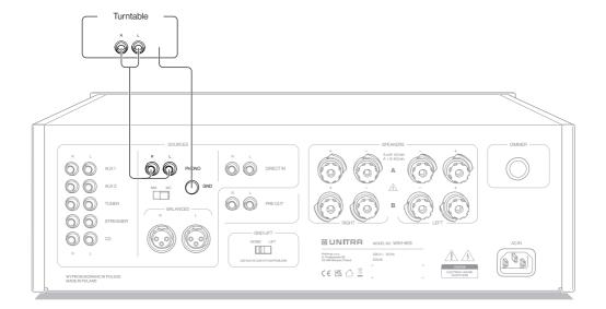
Use the SOURCE selector switch to select the turntable as the input source. 🕒 p. 6.
